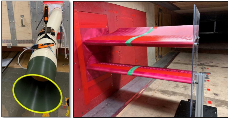
Figure 3. (left) Inlet duct (outside the tunnel) with choke section for load measurements, and (right) 0.5 m chord AeroMINE pair mounted on the wall inside the NWI wind tunnel. This shows the full-height test with a static pressure measurement section (green) mounted between two half-length sections.
