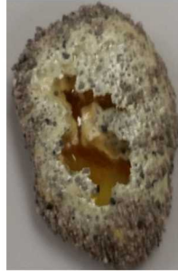
Fig. 5 5F Test sample (dolomite) after cool
