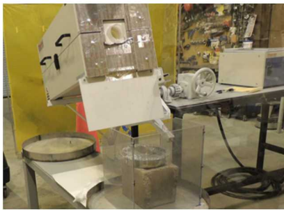
Fig. 5 Apparatus of a tube furnace connected to a crank for pouring onto a catch pan
