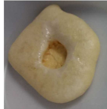
Fig. 3 1E Test Sample used in the porosity determination
