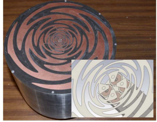
Fig. 3: Prototype four-port sinuous antenna with absorber loaded cavity backing. The inset shows a CAD model of the coaxial cable feed with the substrate hidden to visualize the connection to the antenna arms.
