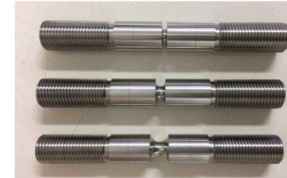
Notched tension specimens and load versus displacement plots
