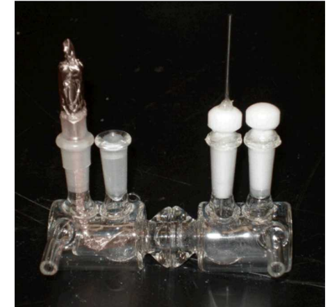
Glass cell used loaded with 25 mol% NaI-AlBr 3 catholyte
