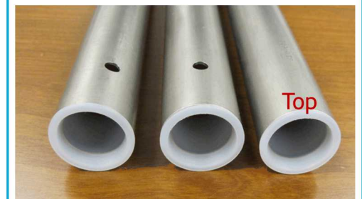
Sleeves ready to be placed in assembly
