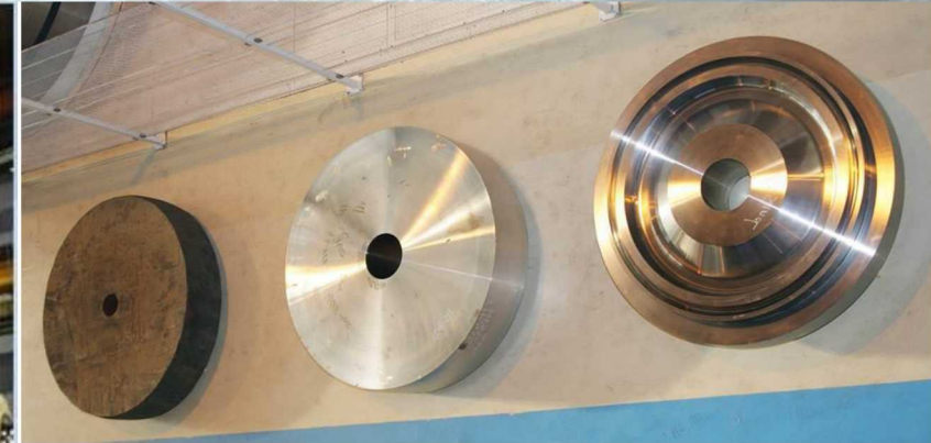
Heavy duty GT rotor disk forging at different manufacturing stage
