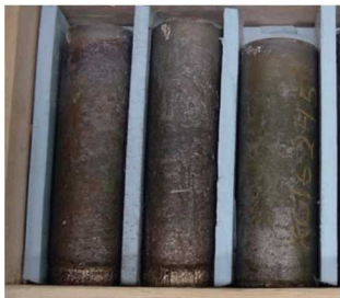
Custom 304L heats created with varying B content
