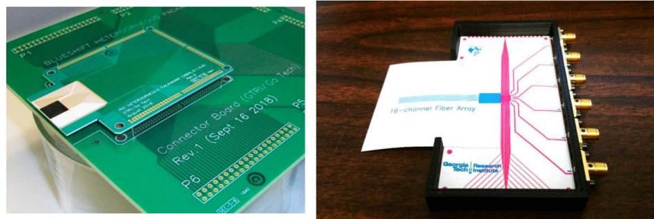
High electrical/RF I/O count photonic integrated circuit packaging.
