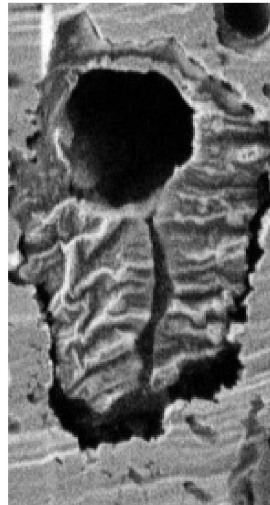
Bitumen-extracted shale with collapsed kerogen
