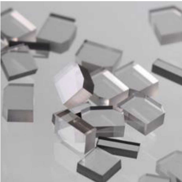
Synthetic diamond chips (few mm)
