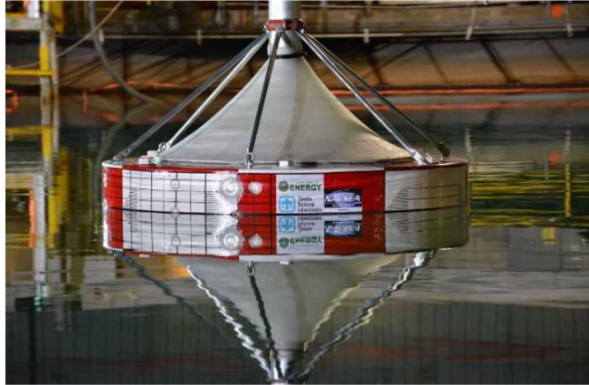
MASK Wave Basin Tests: Increased power absorption by 200%+
