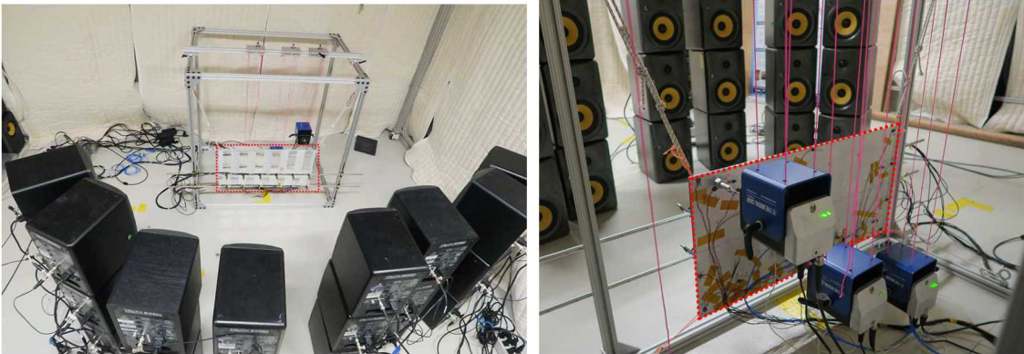
Figure 8: Experiment setups for the acoustic-only “field” test (left) and the combined shaker-acoustic laboratory test (right)
