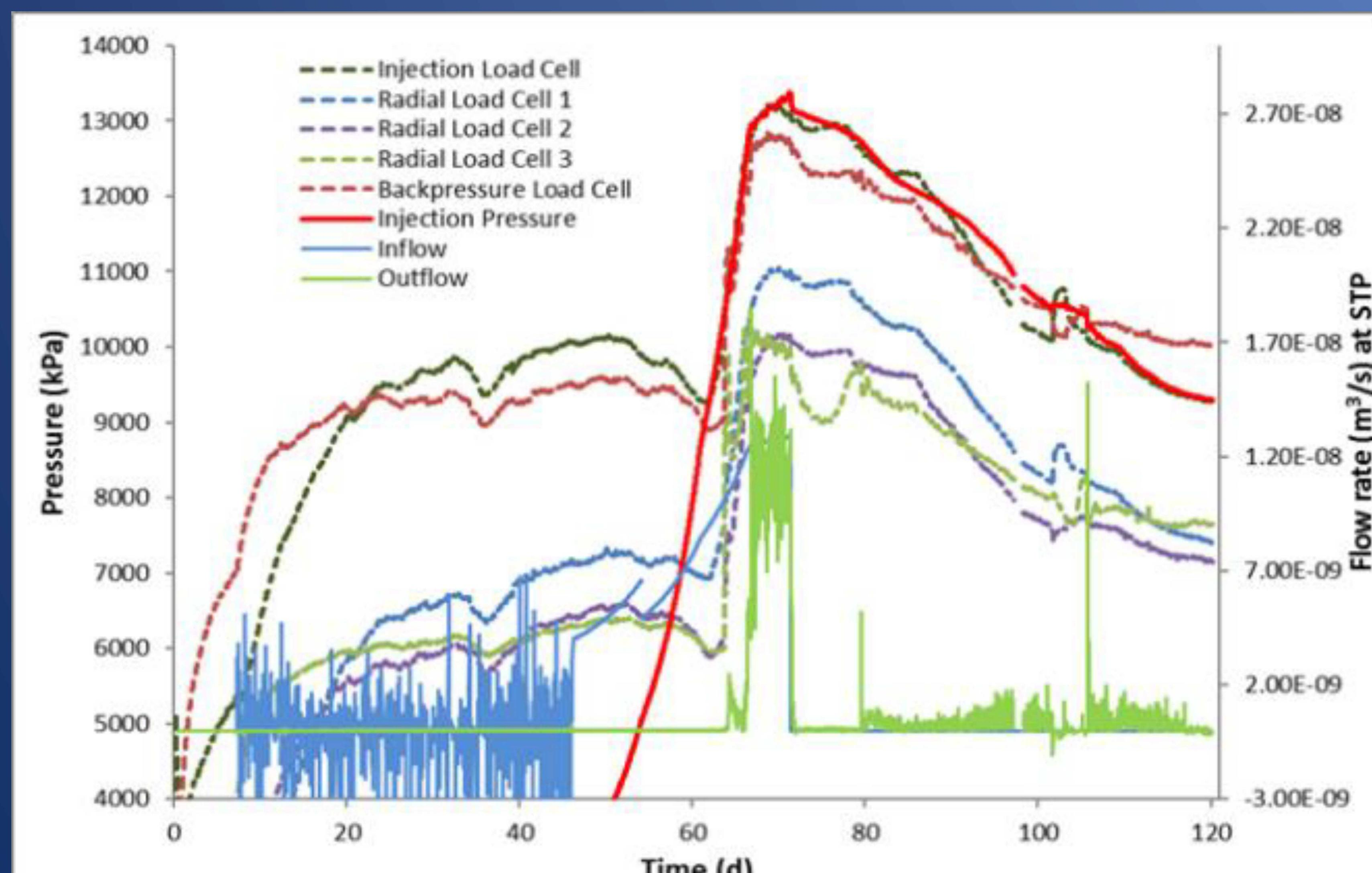
Experimental setup and measurements of gas inflow and outflow rates in water-saturated compacted bentonite Mx80-D.
