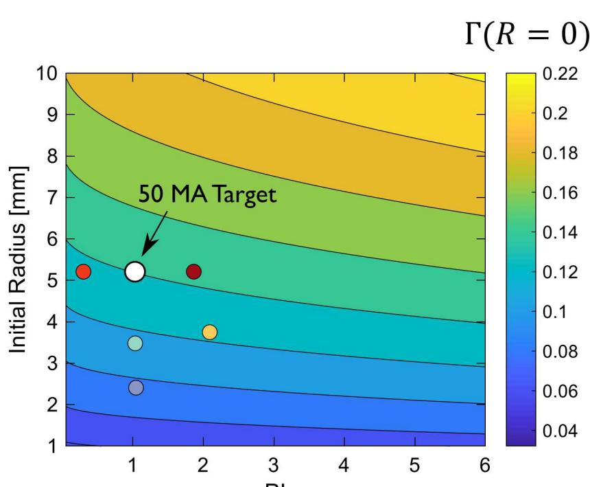
The growth function at peak compression ( $R=0$ ) is plotted and compared to calculated values for select experiments. A notional 50 MA target is highlighted.
