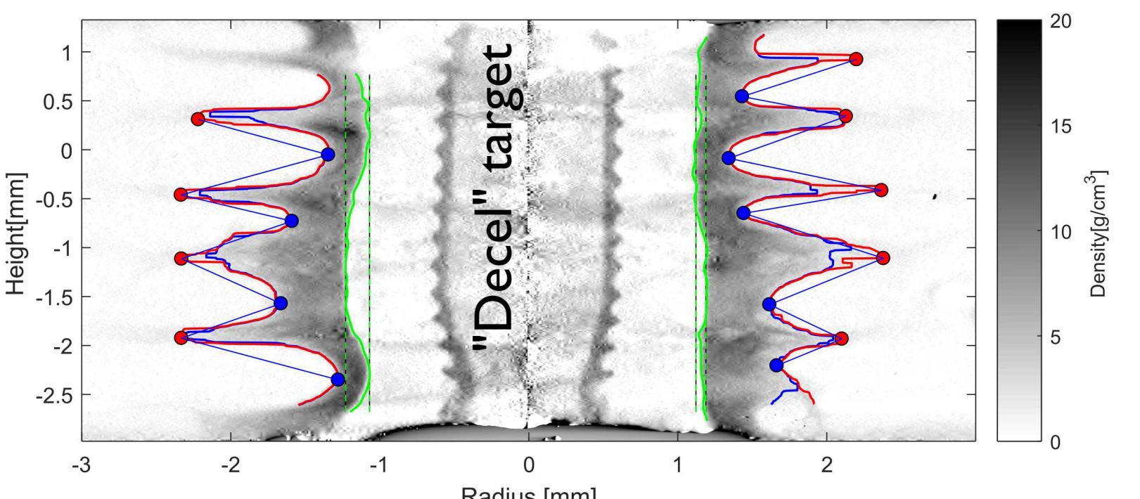
Note: Transmission images were Abel inverted to obtain density maps. The areal-density threshold for contour tracking was typically  $0.5 \cdot (\rho R)_{\text{initial}}$ .
