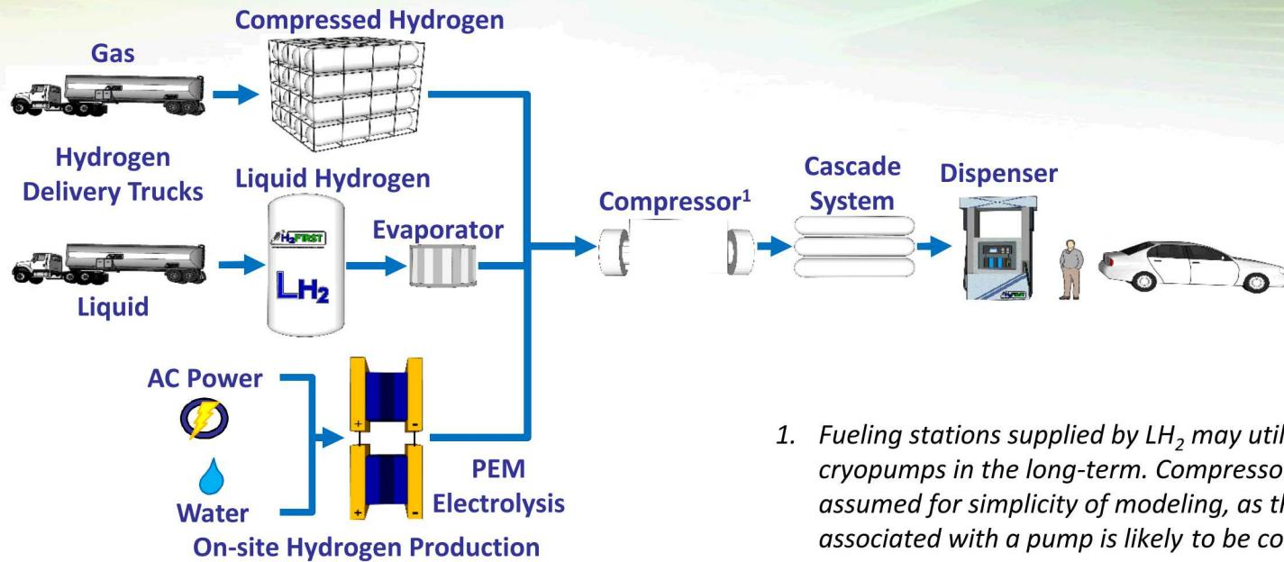
1. Fueling stations supplied by LH<sub>2</sub> may utilize cryopumps in the long-term. Compressors were assumed for simplicity of modeling, as the footprint associated with a pump is likely to be comparable.
