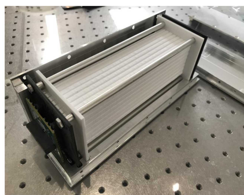
Optically-segmented single volume scatter camera prototype at University of Hawaii (photo credit: N. Kaneshige)
