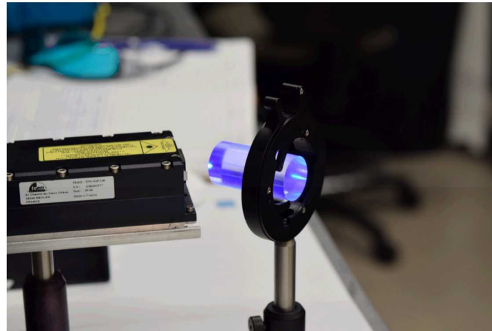
Light spreading effects in bulk plastic scintillator
