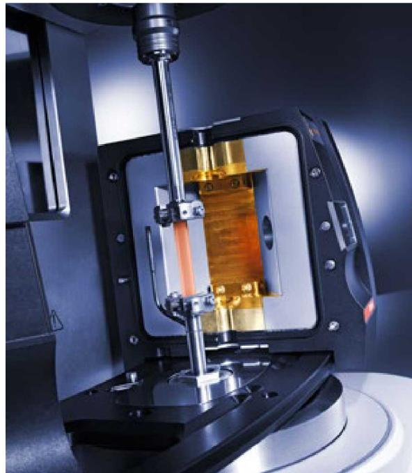
Rectangular torsion geometry measures shear moduli
