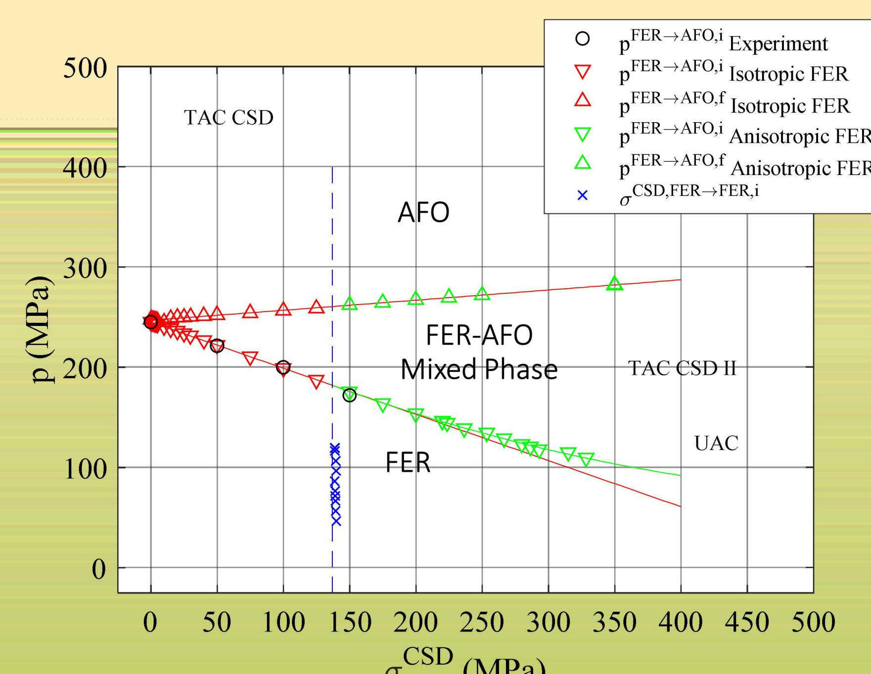
The modeling approach is capable of closely capturing the triaxial loading response of PZT95/5 including the FER and AFO elastic response, the transformation strain under both hydrostatic and triaxial loading, the initiation and termination stress states for phase transformation, and the initiation stress for domain reorientation.
