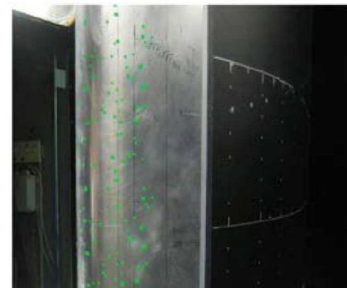
Low- k leading edge laminar/turbulent flow state
