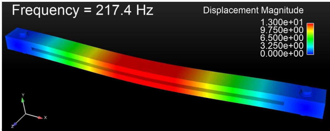
Figure 2. First in-phase bending mode of the linearized beam at 217.4 Hz.
