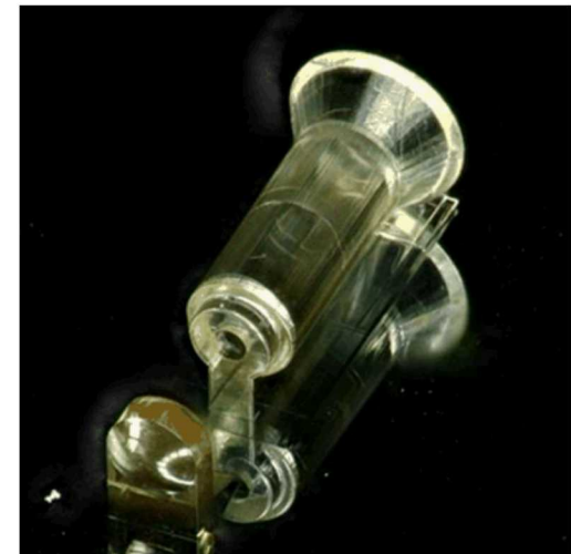
3D printed fiber holder and collimating lens
