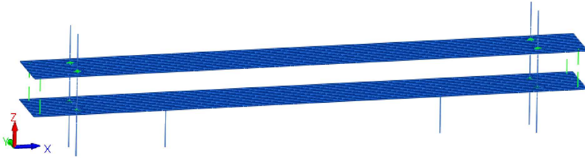
Figure 5. Finite element model of the test structure.
