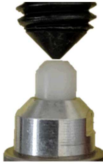
Figure 18. Close-up picture of the nonlinear gap that acts as a contact point when the structure is excited
