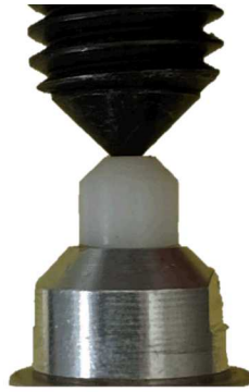
Figure 23. Close-up picture of the nonlinear preloaded contact point
