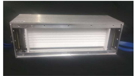
Figure 2. The optically segmented Single-volume scatter camera prototype.
