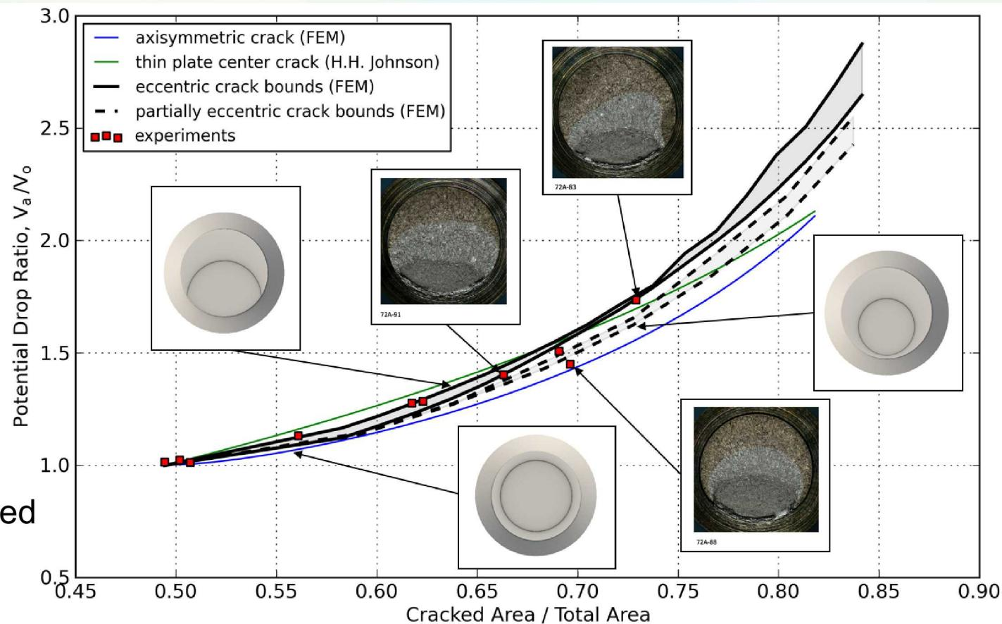
Polynomial relationship between cracked area and DCPD signal provides crack growth information
