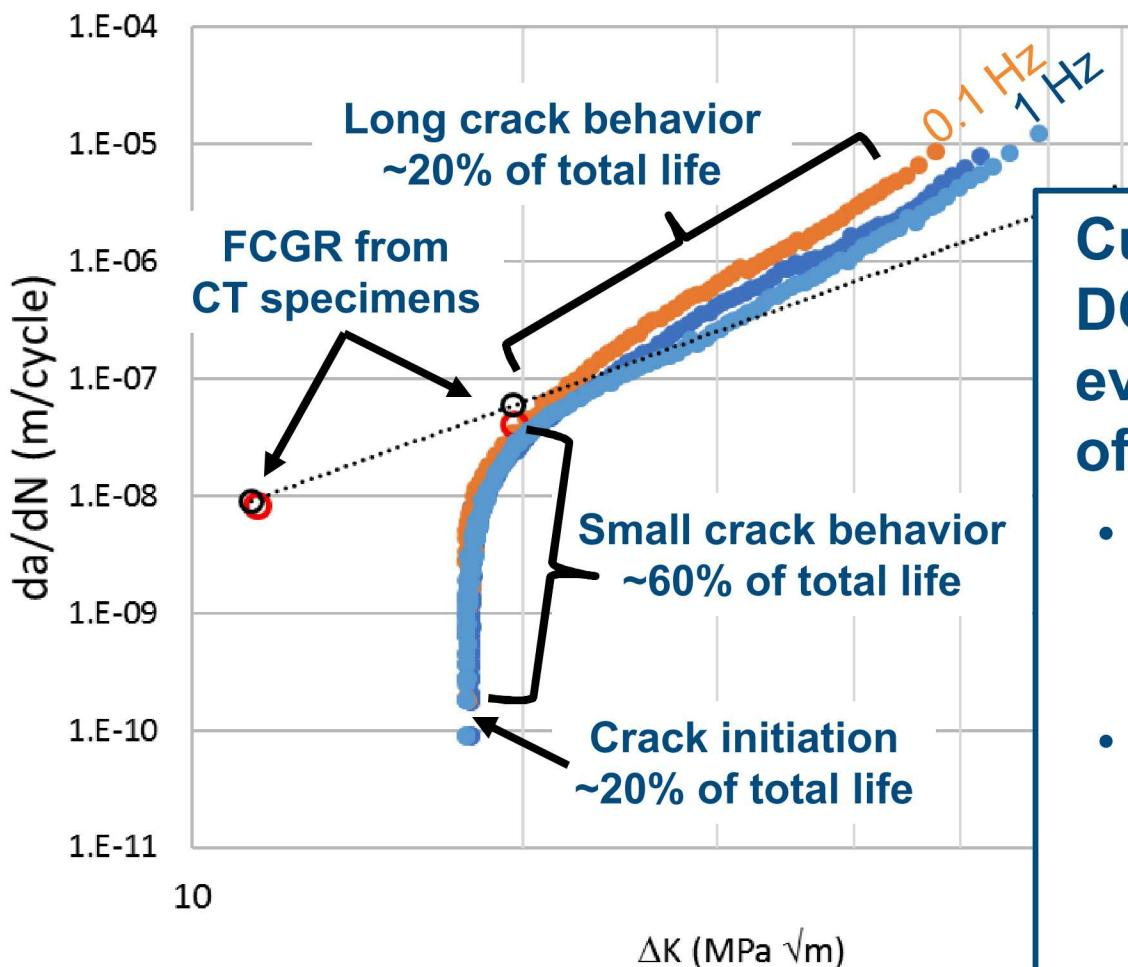
Curves are derived from DCPD data to track crack evolution during fatigue of notched specimens
