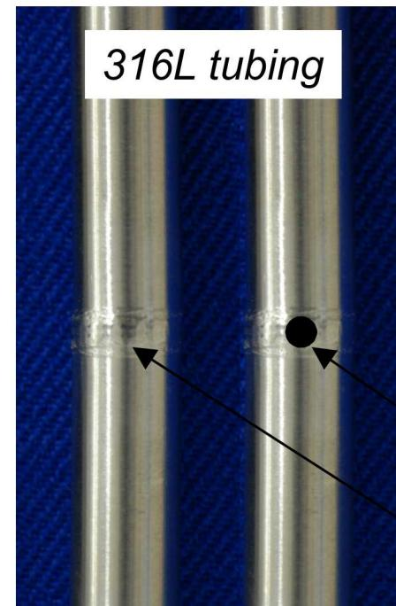
Hole-drilled tube is ideal for evaluation of common weld configuration, such as orbital tube weld
