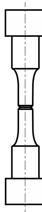
Hole-drilled tubular fatigue specimen
