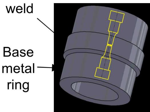
Notched bar is easily applied to large welds, such as GTA welds and EB welds
