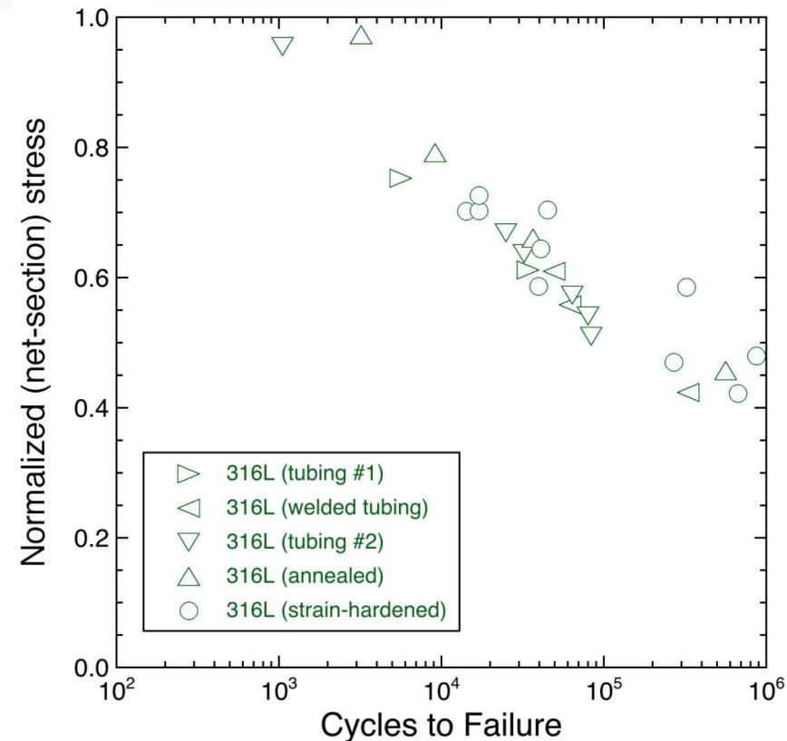
Orbital tube welds behave similarly to base materials in the hole-drilled tube configuration
