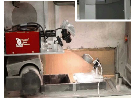
Stratronics ThermaViz 2- color pyrometer installed in ProX 200
