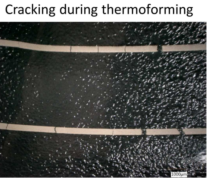
Cracking during thermoforming
