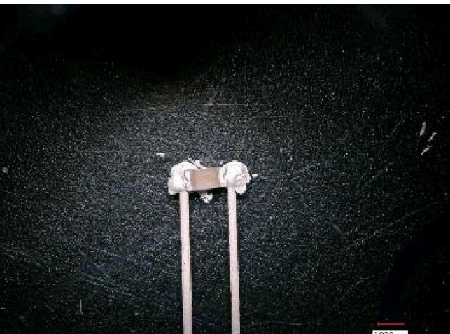
LED attached using conductive adhesive
