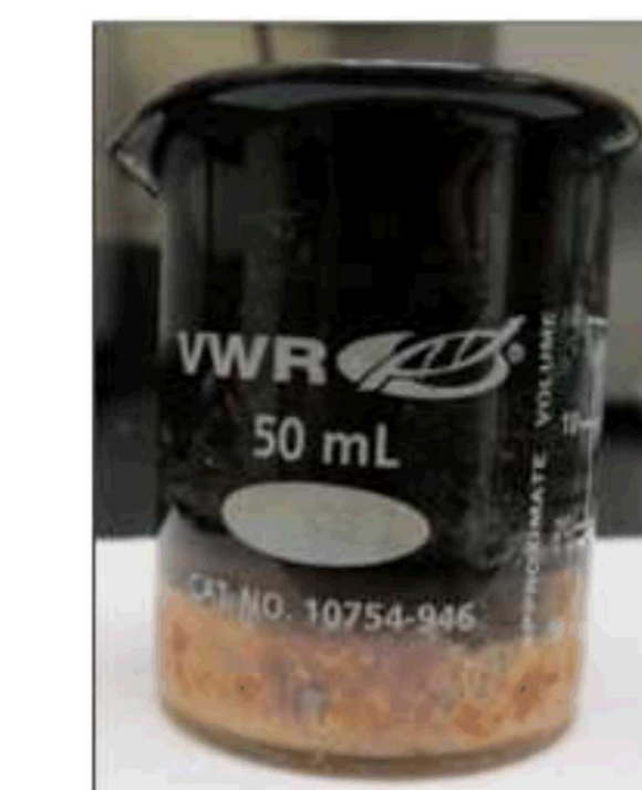
Results of liquid-matrix pyrolysis tests on lutetium nitrate
