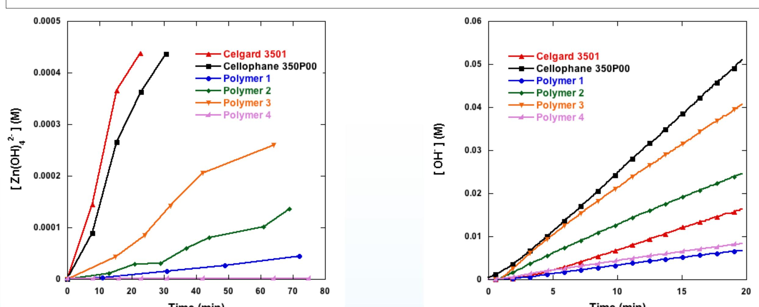
Polymers 1-3 show a greatly improved selectivity ratio over commercial separators for screening out zincate, while allowing for hydroxide crossover. Polymer 4 has an even higher selectivity ratio, but is also far less conductive, resulting in lower practical cycling rates.
