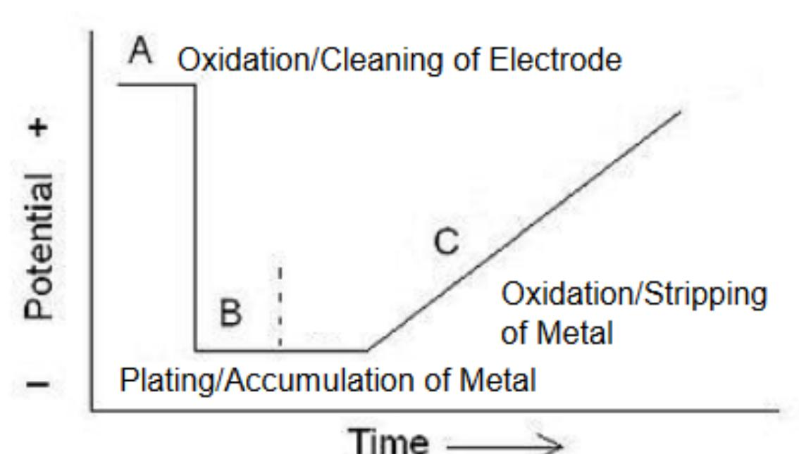
Anodic stripping voltammetry (ASV) allows for much faster screening of separators compared to ICP-MS, with similar limits of detection.
