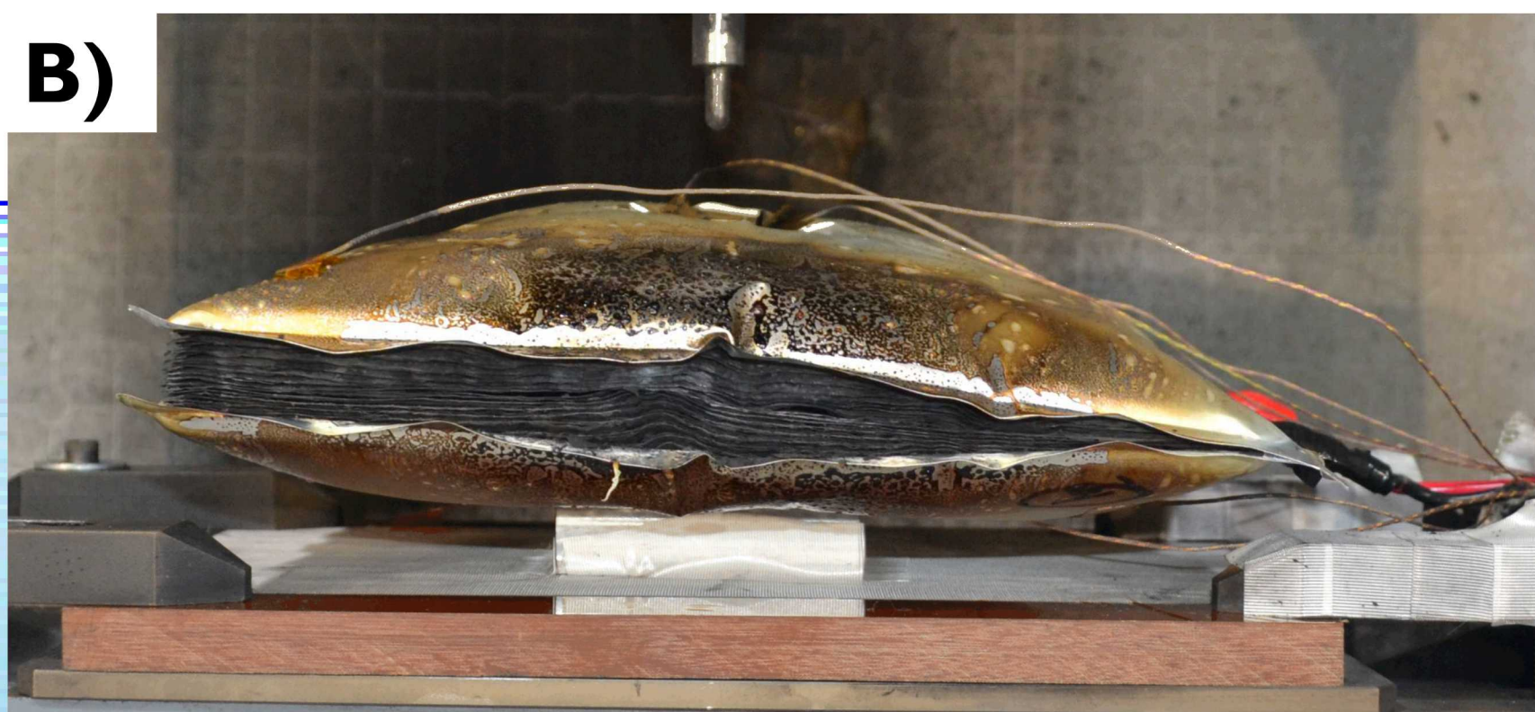
Image 3: A) Post-test Indenter hole of the 50% SOC cell B) Side view of cell swelling and seam separation, showing interior contents
