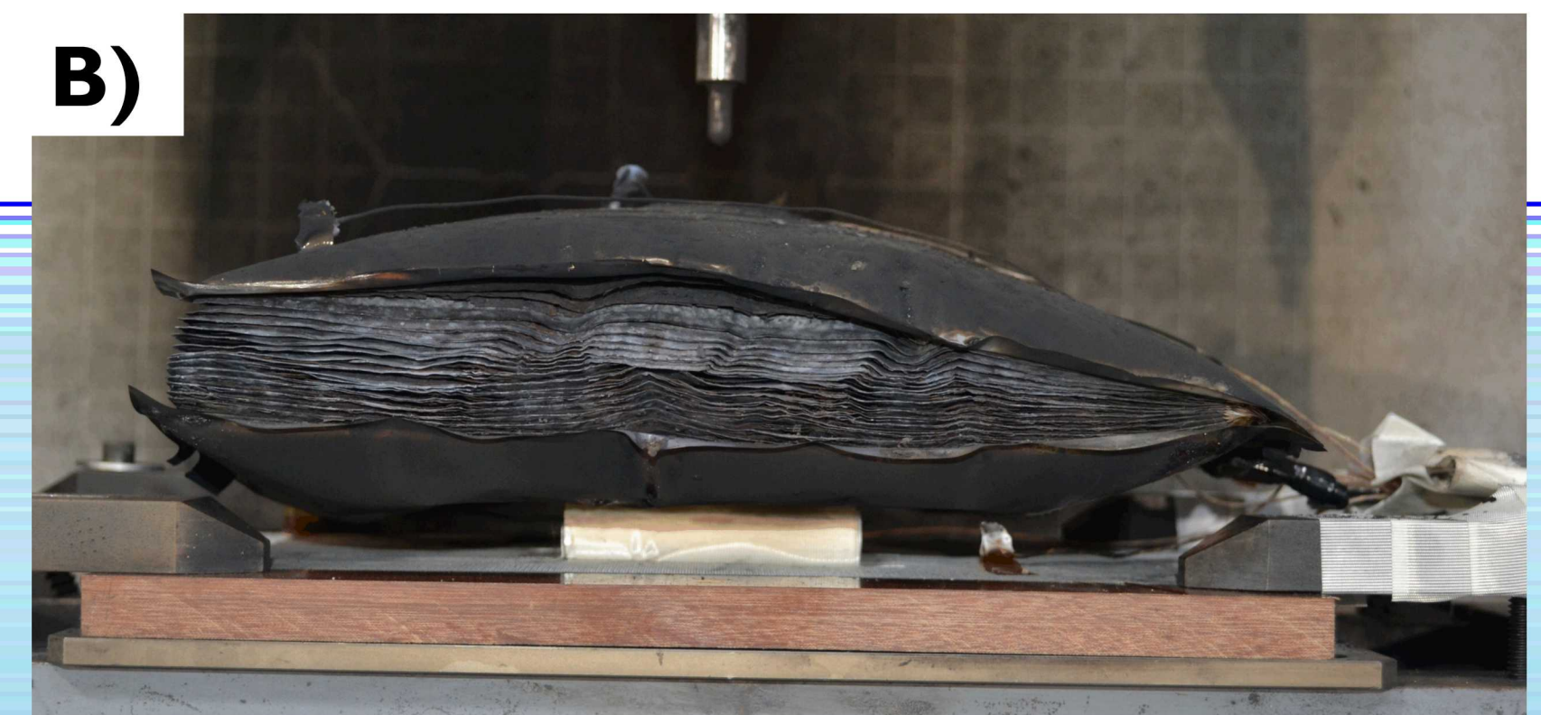
Image 4: A) Post-test Indenter hole of the 75% SOC cell B) Side view of cell swelling, charring and seam separation showing interior contents
