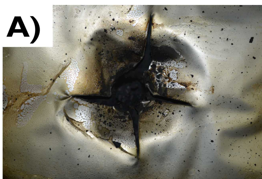
Image 3: A) Post-test Indenter hole of the 50% SOC cell B) Side view of cell swelling and seam separation, showing interior contents
