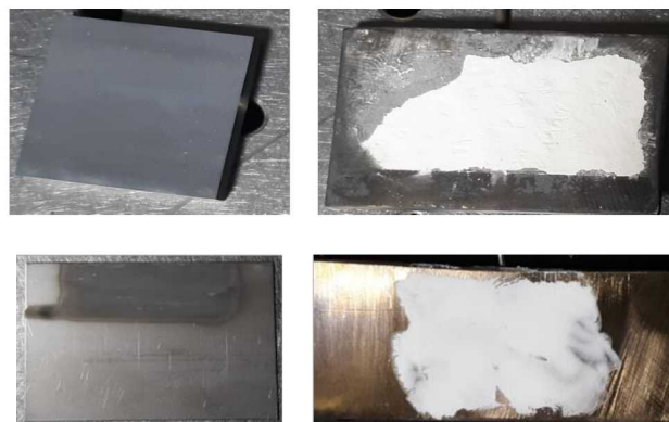
Figure 3. Stainless steel samples. (Top left) Aerosol Deposited YAG:DY. (Top right) “Painted-on” YAG:DY. (Bottom left) Aerosol Deposited MgFGeO:Mn. (Bottom right) “Painted-on” MgFGeO:Mn.
