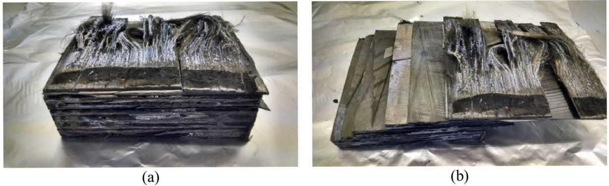
Fig 2: 29 mm sample after being tested in the Cone Calorimeter. (a) shows the block of the sample with carbon fibers oxidized on the surface and the rest of the sample being pyrolysed. (b) shows the different layers of carbon fiber detached after pyrolysis.
