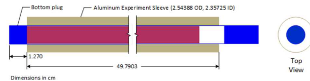
Fuel Element with Aluminum Sleeve
