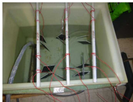
Fig. 5. Test setup for metal-carbon fiber composite interconnects at Florida Atlantic University.
