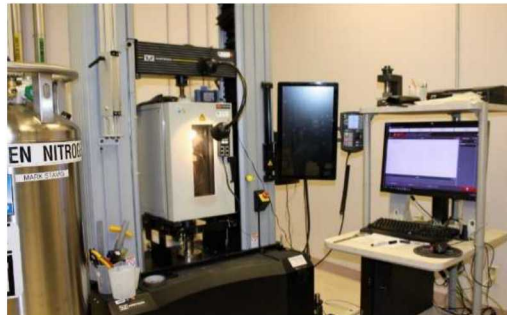
FIGURE 4. Instron hoop stress test setup.
