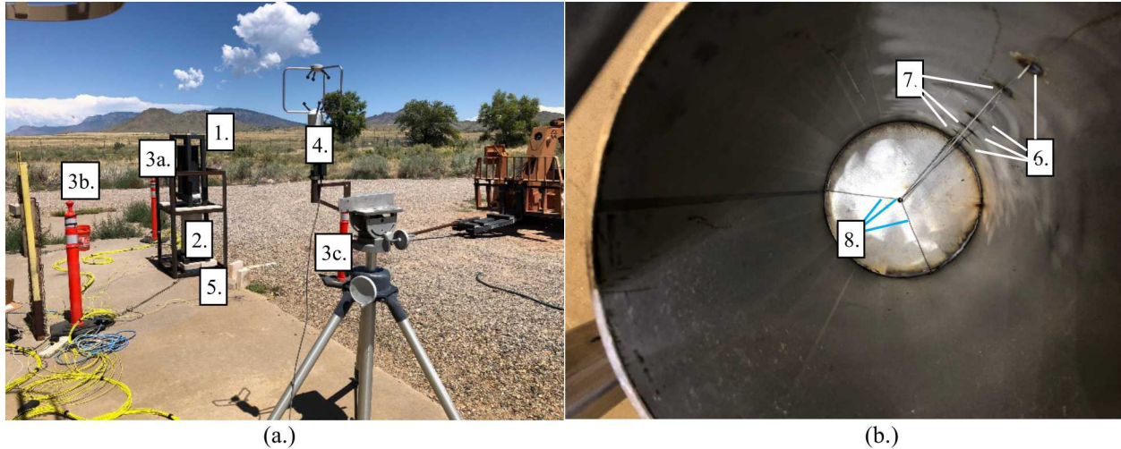
Figure 8. (a.) Test configuration: 1, hot particle test bin. 2, catch bin. 3a-c, ambient thermocouples. 4, anemometer. 5, scale. (b.) Thermocouple placement: 6, wall TCs 1-4 from top to bottom. 7, center TCs 1-3 from top to bottom. 8, outlet TCs 1-3
