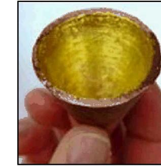
3-D Integrated Gold THz Waveguides
