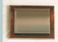
IR Focal Plane Array w/ ROIC
