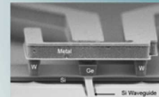
Germanium Detector on Silicon
