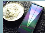
Array Waveguide Grating Channelizing Filter
