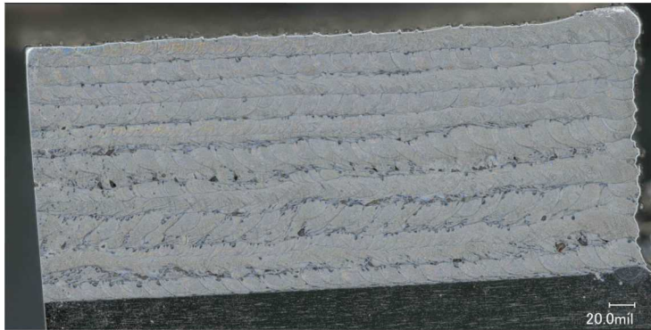
Laser-deposited material displays excellent combination of strength and ductility
