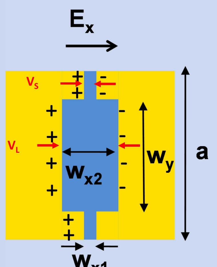
The quasi-static behavior of this structure is non-resonant thus enabling a broadband optical response.
