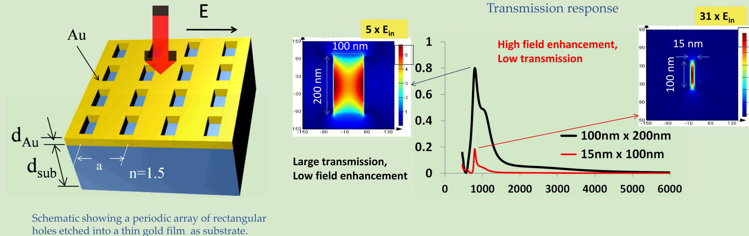
**Operational principle :** Incoming light excites resonant surface plasmon polaritons in the metal due to the periodic hole arrays, causing the electric field to be confined in the subwavelength gap and enabling its transmission.
