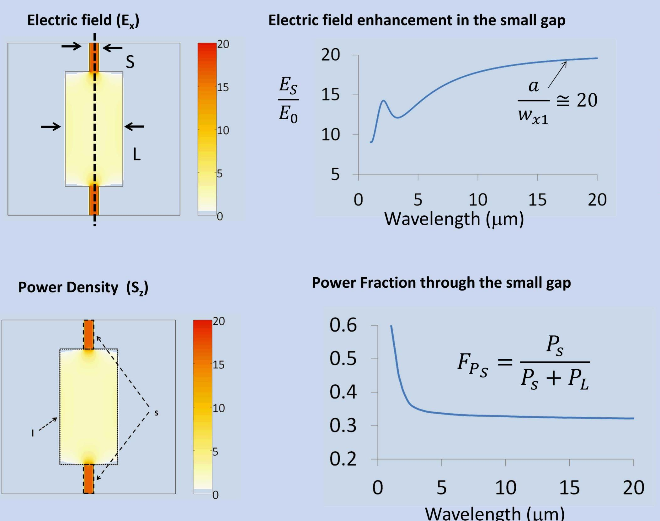
The electric field in the small gap is enhanced across a broad wavelength range approaching an asymptotic value determined by the geometry of the structure.
