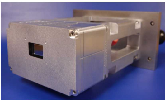
Opacity Spectrometer with 2 UXI Cameras in the Axial Package
