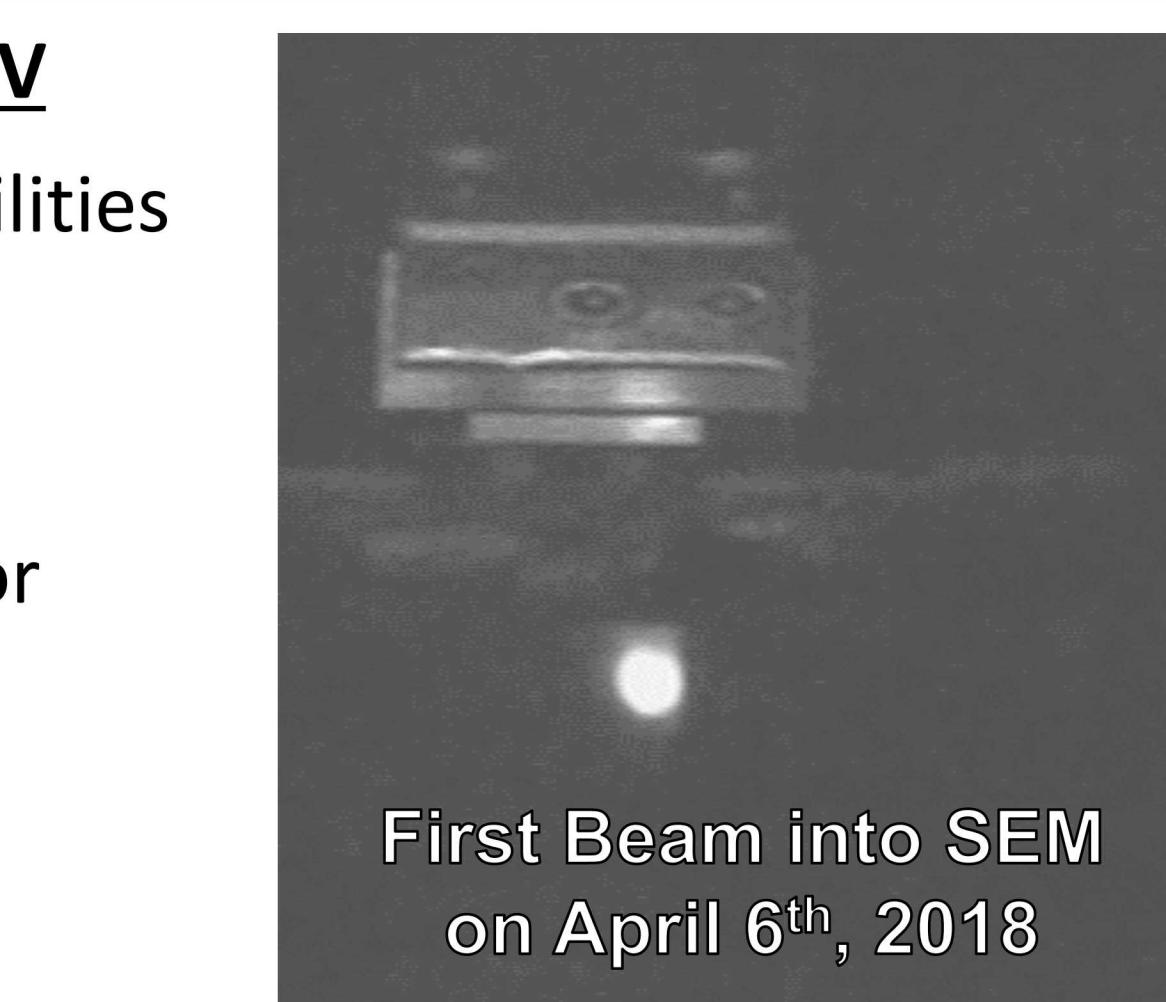
Figure 2: Ion beam induced luminescence (IBIL) on a quartz target in the SEM
