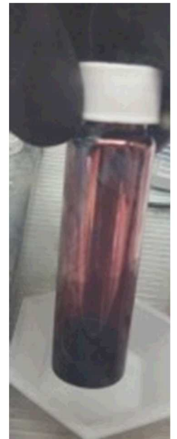
Cu Nanoparticles used to formulate an ink for aerosol jet printing
