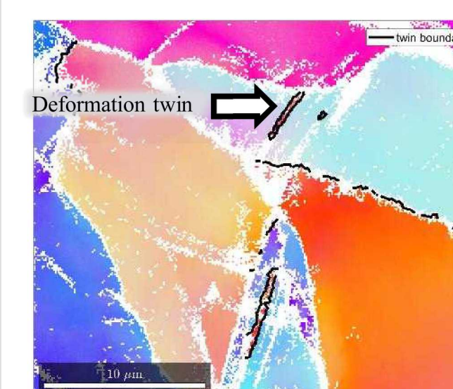
IPF map colored with respect to the STD with twin boundaries overlaid
