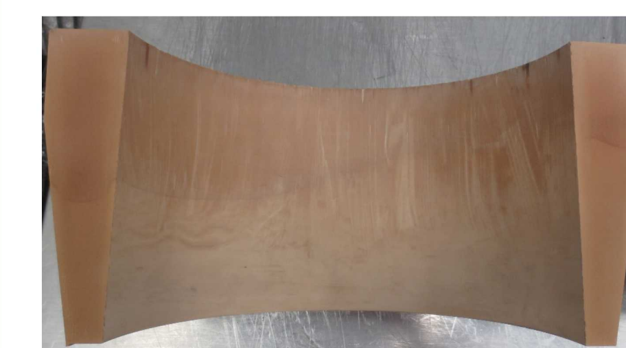
Figure 5. Billet following a two-hour hold at 153.7 °C
