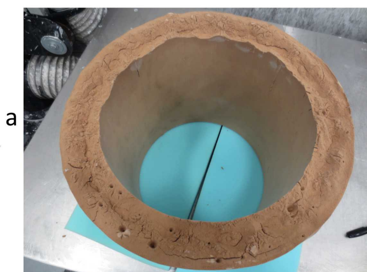
Figure 6. Billet following a 24-hour hold at 153.7 °C
