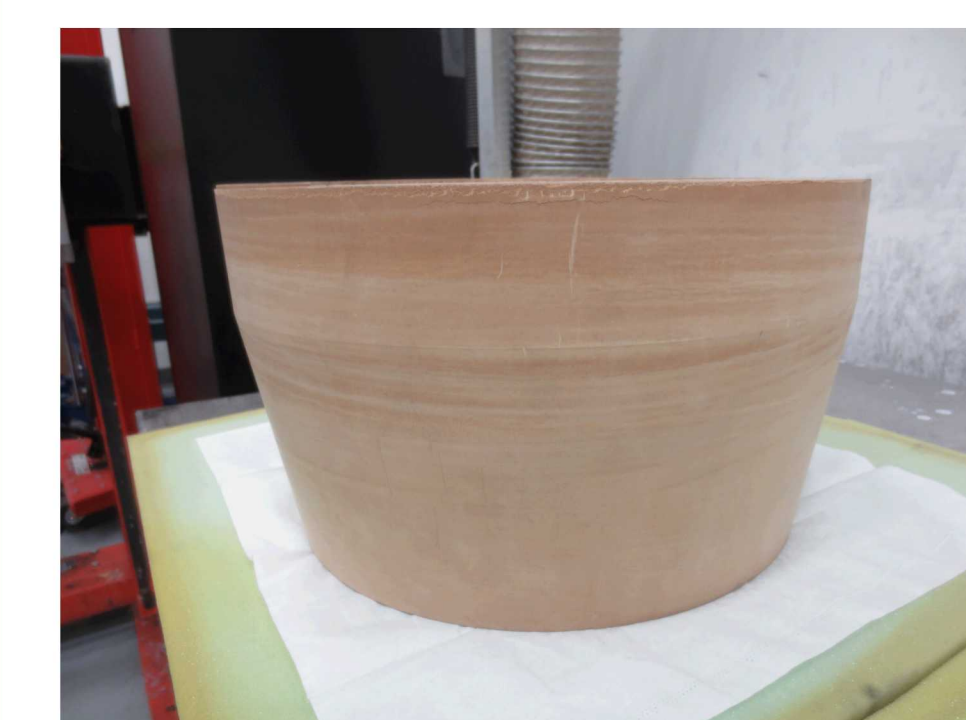
Figure 10. First known single-tone billet at a nominal density of 0.5 g/cc
