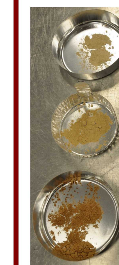
Figure 7. Samples of 070328 (left) heat treated at 70, 110, and 128 °C in descending order from top to bottom and their associated DSC traces.
