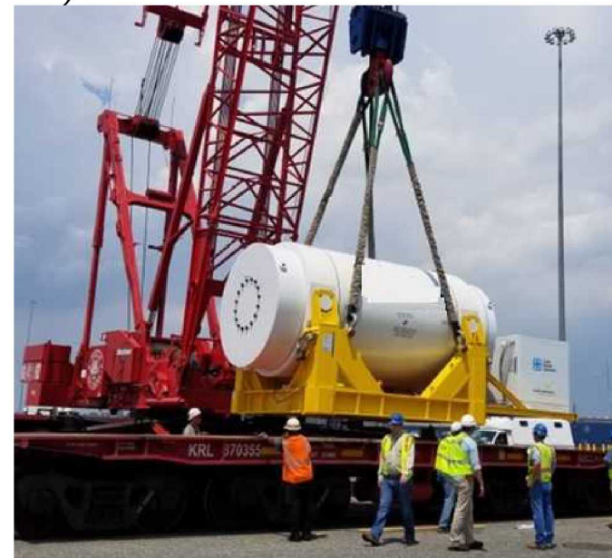
Photo of a mock SNF cask being moved from a container ship to heavy haul truck as part of a multi-modal, multi-jurisdictional international transportation route. Copyright: Sandia National Laboratories.
