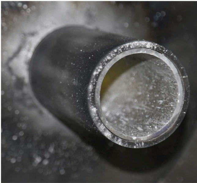
June 2019: (dark) outer sleeve is 1/4 - inch thick 1026 Cold-Rolled Steel
