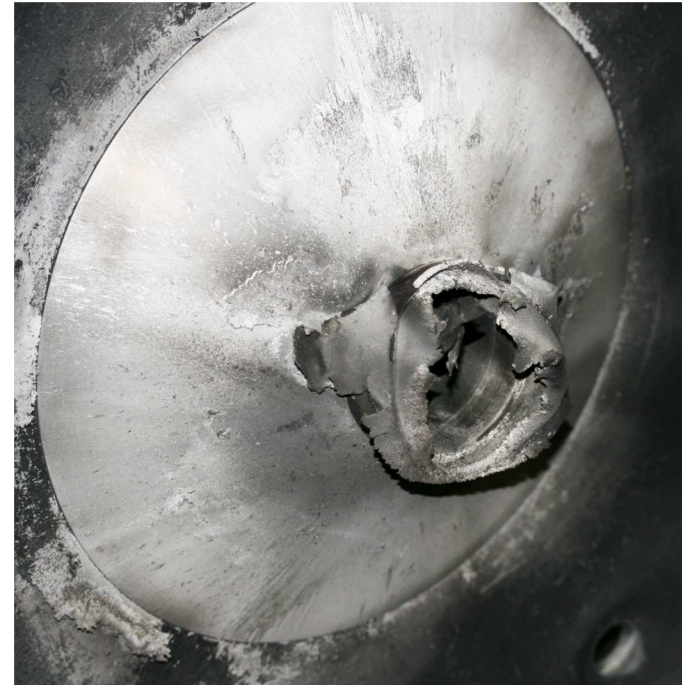
April 2017: (remaining) outer sleeve is 1/8-inch thick aluminum 6061
