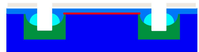
3. Vias are etched through oxide, Si Cap, remaining oxide, and into the implanted region
