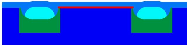
1. Device as it arrives in BEOL after STM
