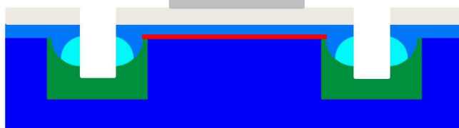
4. Aluminum top gate defined by EBL is deposited over patterned device.
