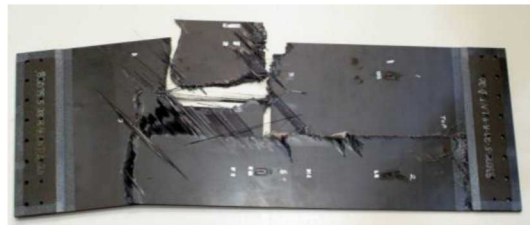
Typical damage progression in a notched composite panel (photo courtesy Boeing)
